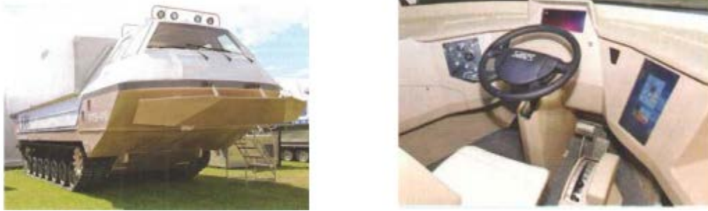
Figure 2 – Floating crawler conveyor search and rescue PTS-PS
