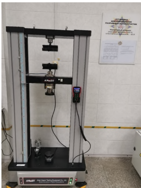
Figure 1. – Installation for determining discontinuous characteristics
