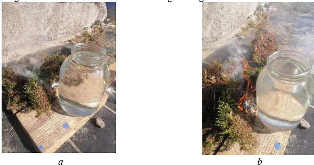
**Figure 1 – Ignition of moss when exposed to focused solar radiation
