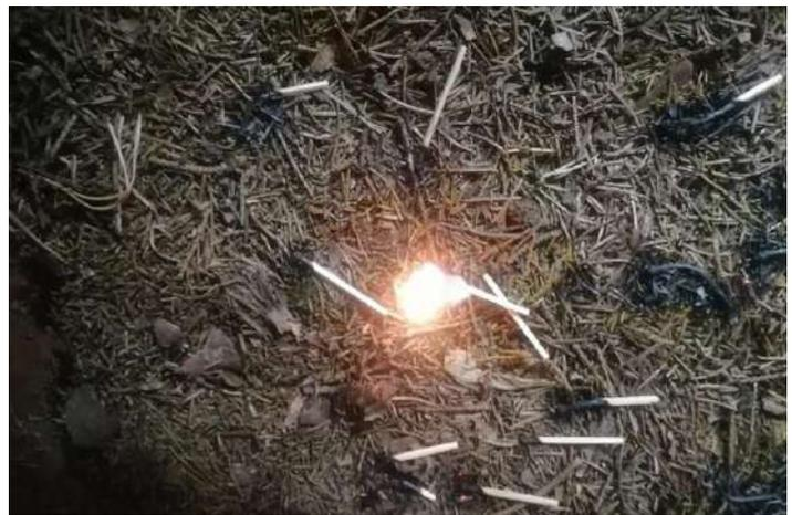
**Figure 2 – The process of exposure of a sample of spruce needles to a burning match without the occurrence of stable flame combustion**
