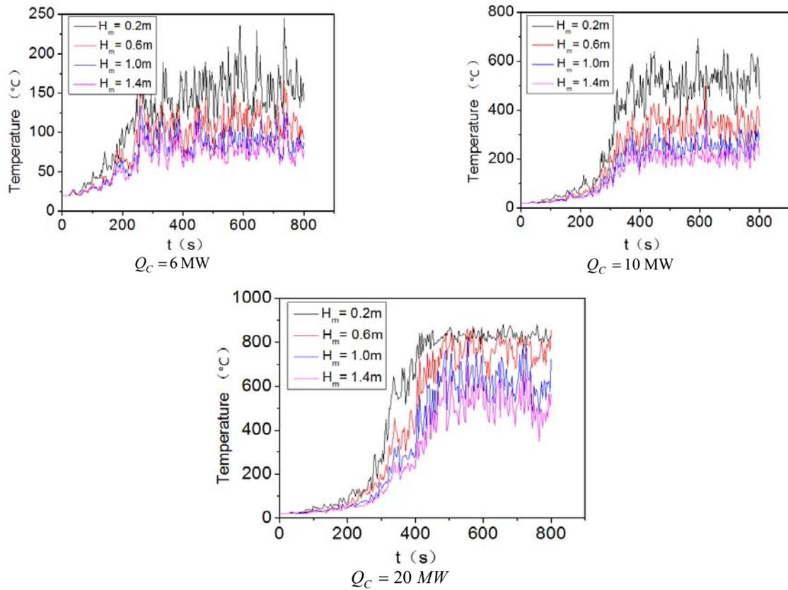
Figure 3. – Temperature curve along the centerline above the upper room window ( $L_{hp} = 0$  m)
