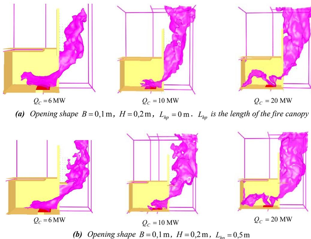
**Figure 2. – Isothermal surface at 250 °C**
