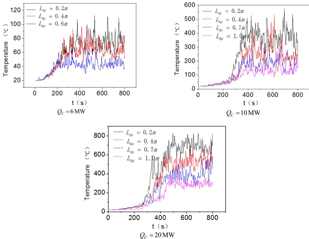
Figure 4. – Temperature curve along the centerline above the upper room window ( $H_m = 0.4$  m)
