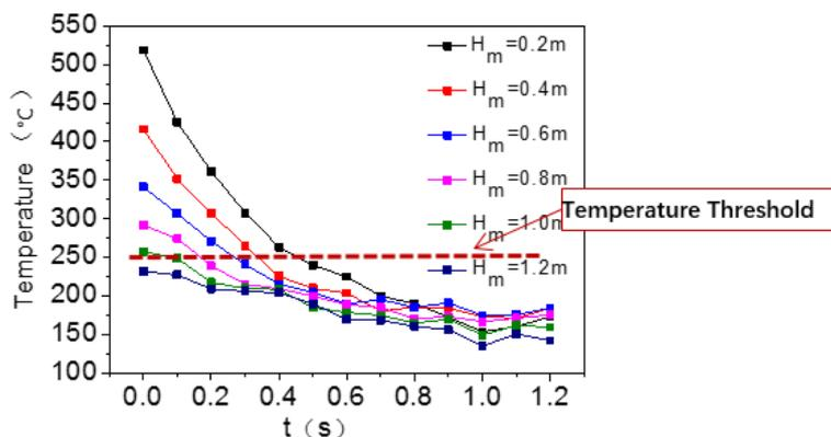
Figure 5. – Temperature distribution of building facade for different fire canopy width and wall height between windows at  $0 < Q_{ex}^* < 1,3$
