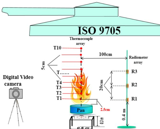
Figure 1. – The experimental arrangement
