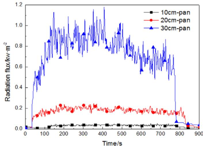
Figure 8. – R2 heat flux density meter measured thermal radiation flux vs time
