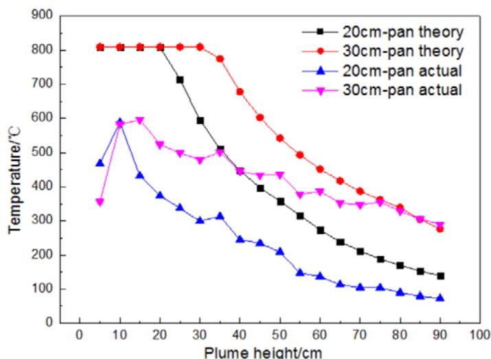
Figure 7. – The flame stability phase axis of the plume temperature contrast
