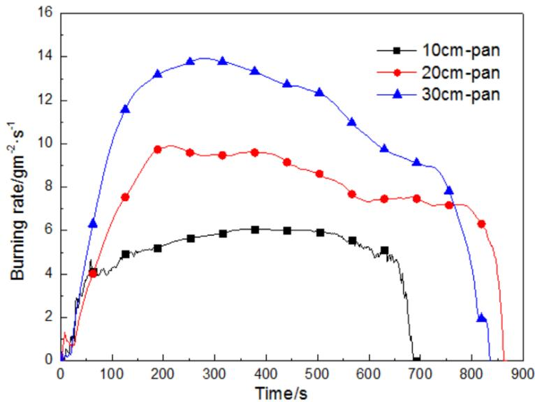
Figure 3. – Relationship between burning rate and time
