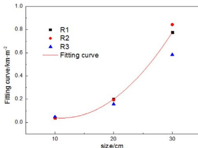
Figure 9. – The thermal radiation flux of different sizes of oil pool and the fitting curve
