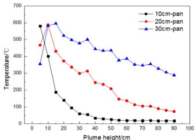
Figure 6. – Different sizes of oil pool steady state temperature vs height
